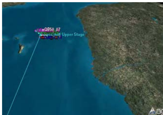
Figure 99: En masse, high recontact risk of hypothetical bunched deployment one orbit after launch
