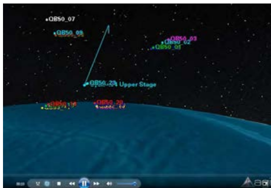
Figure 98: Hypothetical bunched bad deployment, with no thrusting by deployer and little or no inter-satellite relative velocity at deployment
