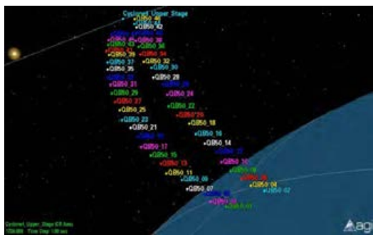
Figure 96: Proposed QB50 deployment under upper stage along-track thrusting
