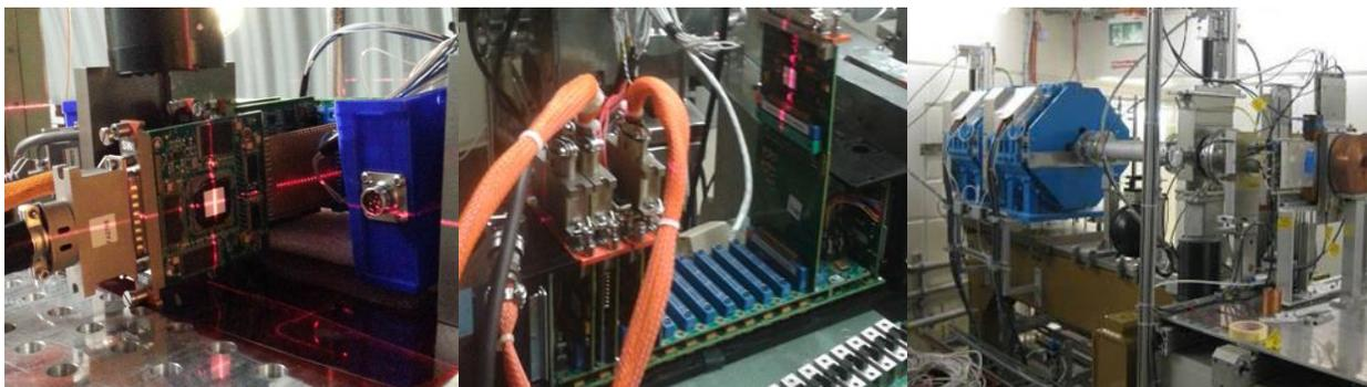
**Exhibit 7:** KAM-500 module hosted in KAM-500 Smart Backplane chassis during the radiation tests
