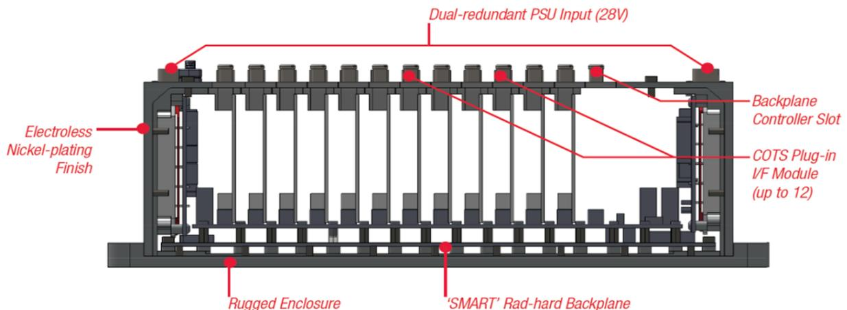
**Exhibit 4:** Cross-section of KAM-500 Smart Backplane chassis populated with plug-in modules
