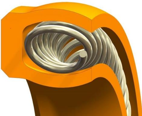
**Figure 4 - APS Seal Type (Advanced Pitch Spring) - produces almost constant spring load over a wide range of deflection. Good for high speed service.**
