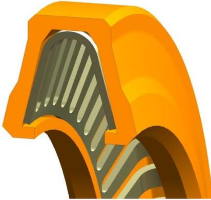
**Figure 5 - RACO Face Seal Type - Ideal for cryogenic service with extremely low leakage requirement. Continuous edge spring provides uninterrupted edge sealing and minimizes seal jacket shrinkage.**
