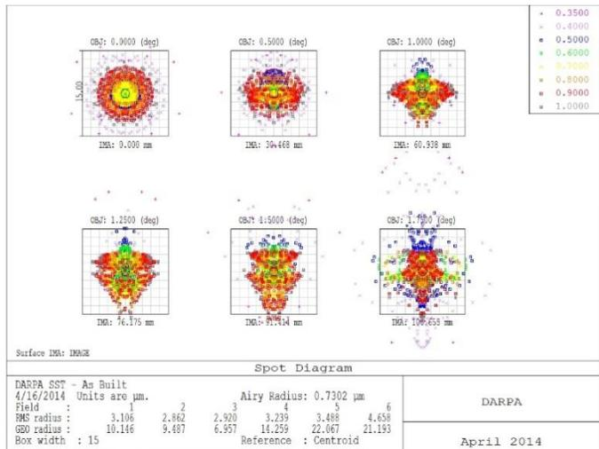
**Exhibit 9. SST spot diagram. The boxes are representative of the actual 15 $\mu\text{m}$  pixels.**
