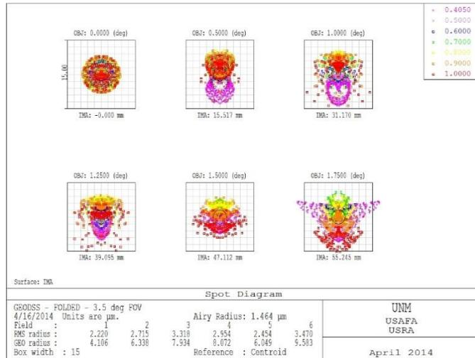
**Exhibit 12.** Spot diagram for wide-field GEODSS upgrade. The boxes are representative of the recommended  $15\mu\text{m}$  pixels.
