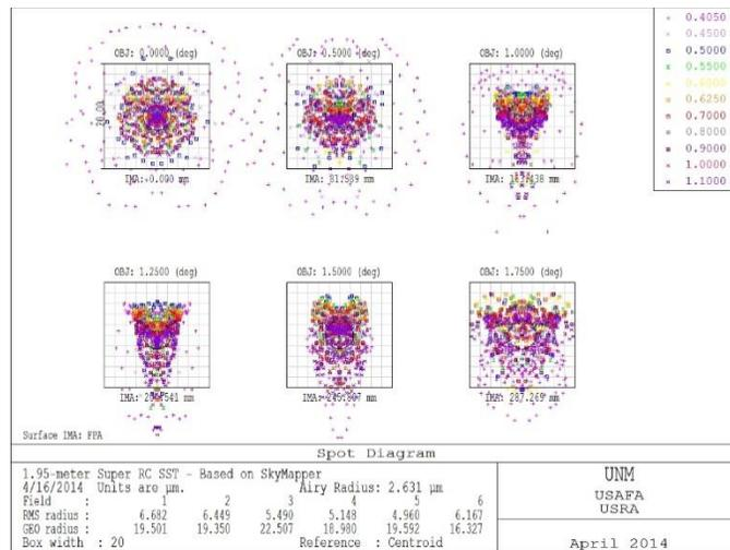
**Exhibit 18.** Spot diagram for 1.95-m SkyMapper. The boxes are representative of the recommended 20 $\mu\text{m}$  pixels.
