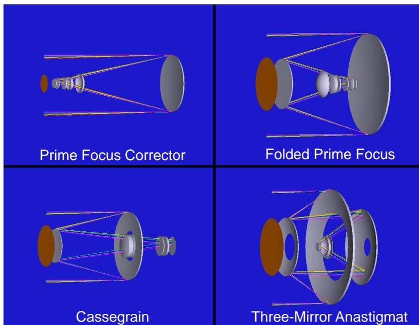
**Exhibit 3.** Optical layout options. The red disk seen on each layout shows the extent of the central obscuration.
