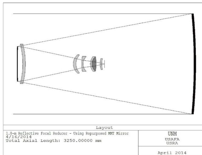
**Exhibit 20.** Optical layout for repurposed MMT mirror.
