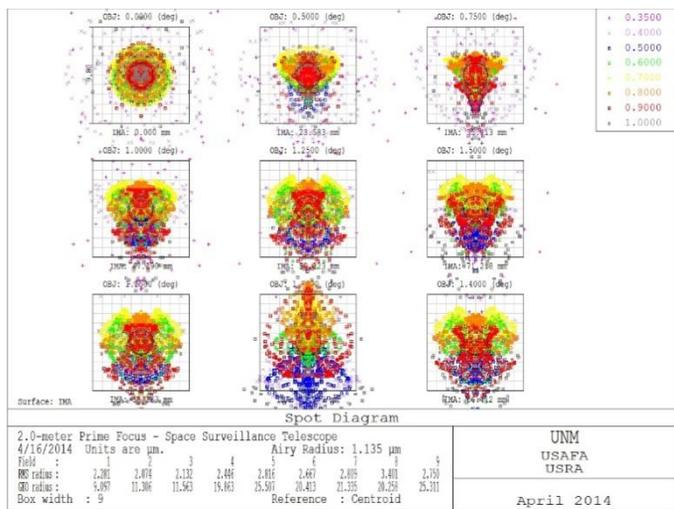
**Exhibit 24.** Spot diagram for 2.0-m prime focus system. The boxes are representative of the recommended 9 $\mu\text{m}$  pixels.
