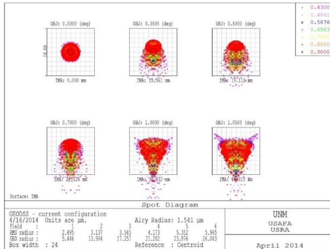
**Exhibit 6.** GEODSS spot diagram. The boxes are representative of the actual 24 $\mu\text{m}$  pixels.
