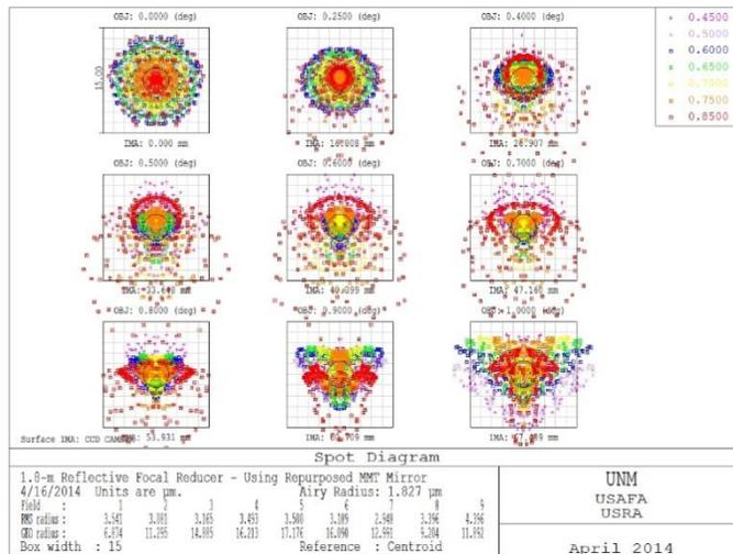
**Exhibit 21.** Spot diagram for repurposed MMT mirror. The boxes are representative of the recommended 15 $\mu\text{m}$  pixels.
