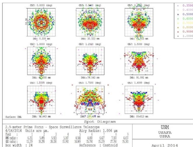
**Exhibit 27.** Spot diagram for 2.9-m prime focus system. The boxes represent 24 $\mu\text{m}$  pixels.
