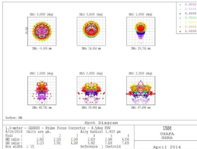
**Exhibit 15.** Spot diagram for very wide-field GEODSS upgrade. The boxes are representative of the recommended  $15\mu\text{m}$  pixels
