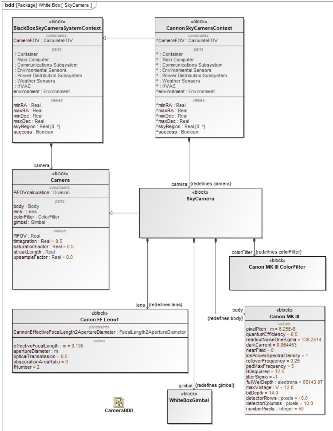
**Figure 10:** This diagram shows the specification of a camera design from the 'abstract' camera model. The specific camera components can then be defined as shown to allow multiple configurations to be specified from the base design. This approach enables the engineer to assess individual performance or optimize parameters during a Multi-Disciplinary Analysis and Optimization study.
