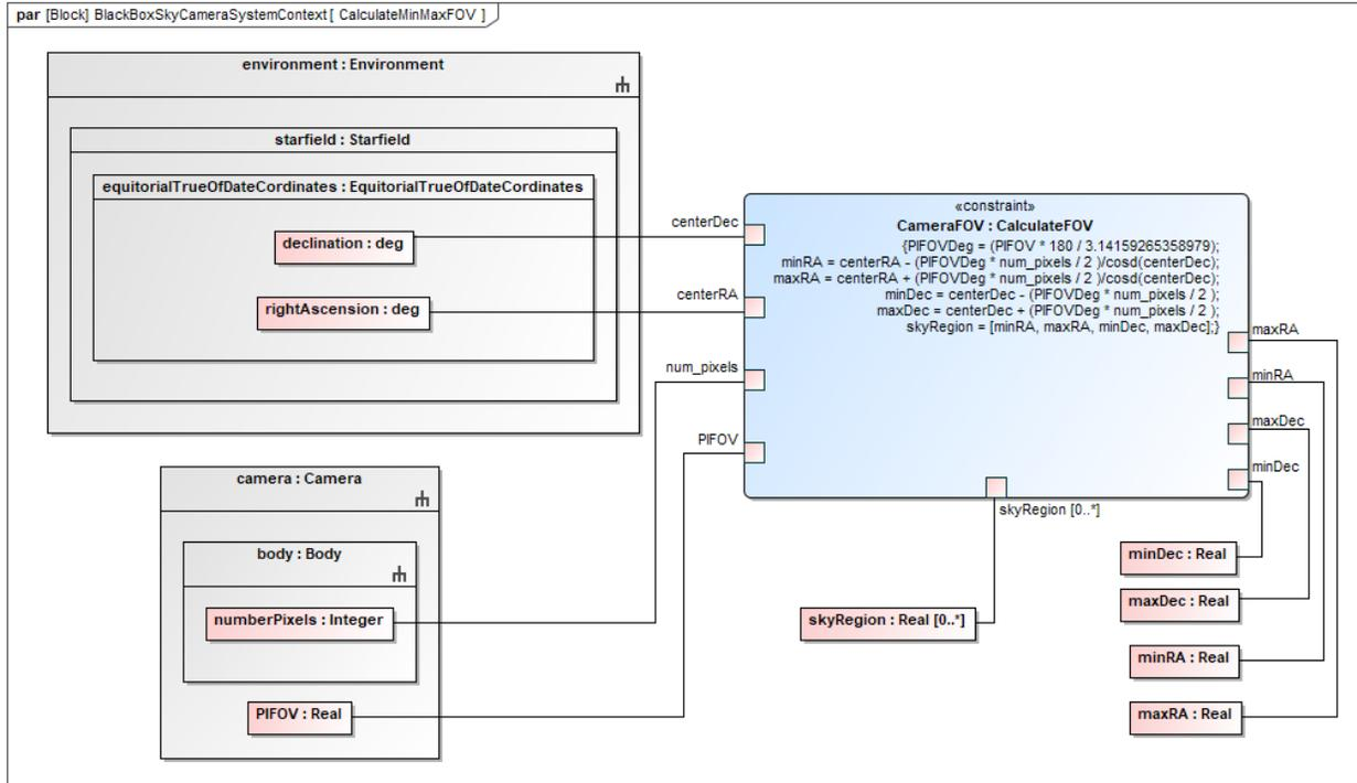
**Figure 5:** Example of MATLAB code as a parametric constraint for the field of view calculation.
