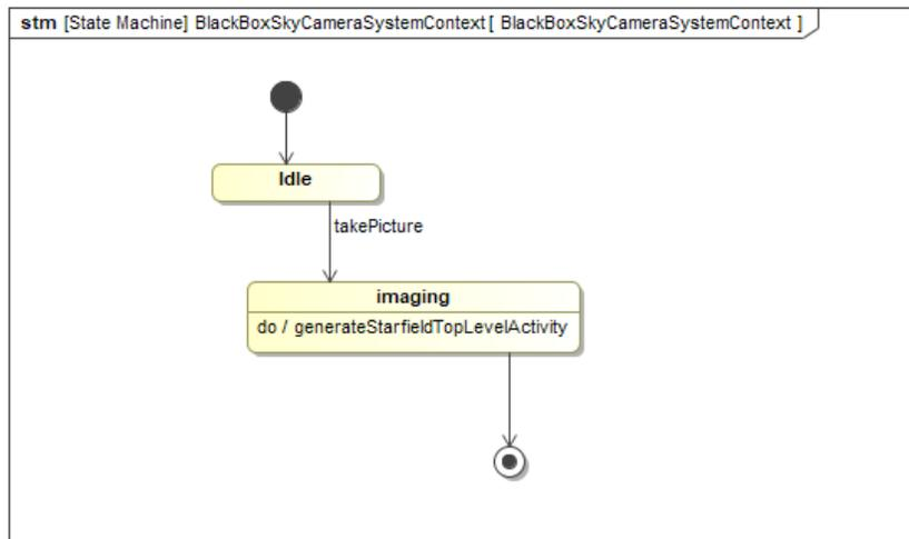
**Figure 7:** This is the classifying behavior of the BlackBoxCameraSystemContext block. The system model starts in an idle state to allow the user to set camera parameters before signaling the camera to ‘take a picture.’
