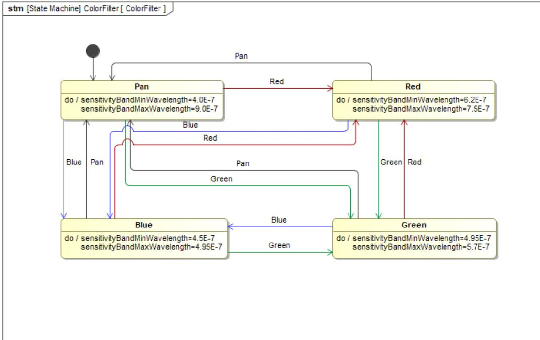
**Figure 6:** A state machine that shows the color filter classifying behavior. We used a similar state machine to select the star catalog and to model the camera tracking gimbal states.
