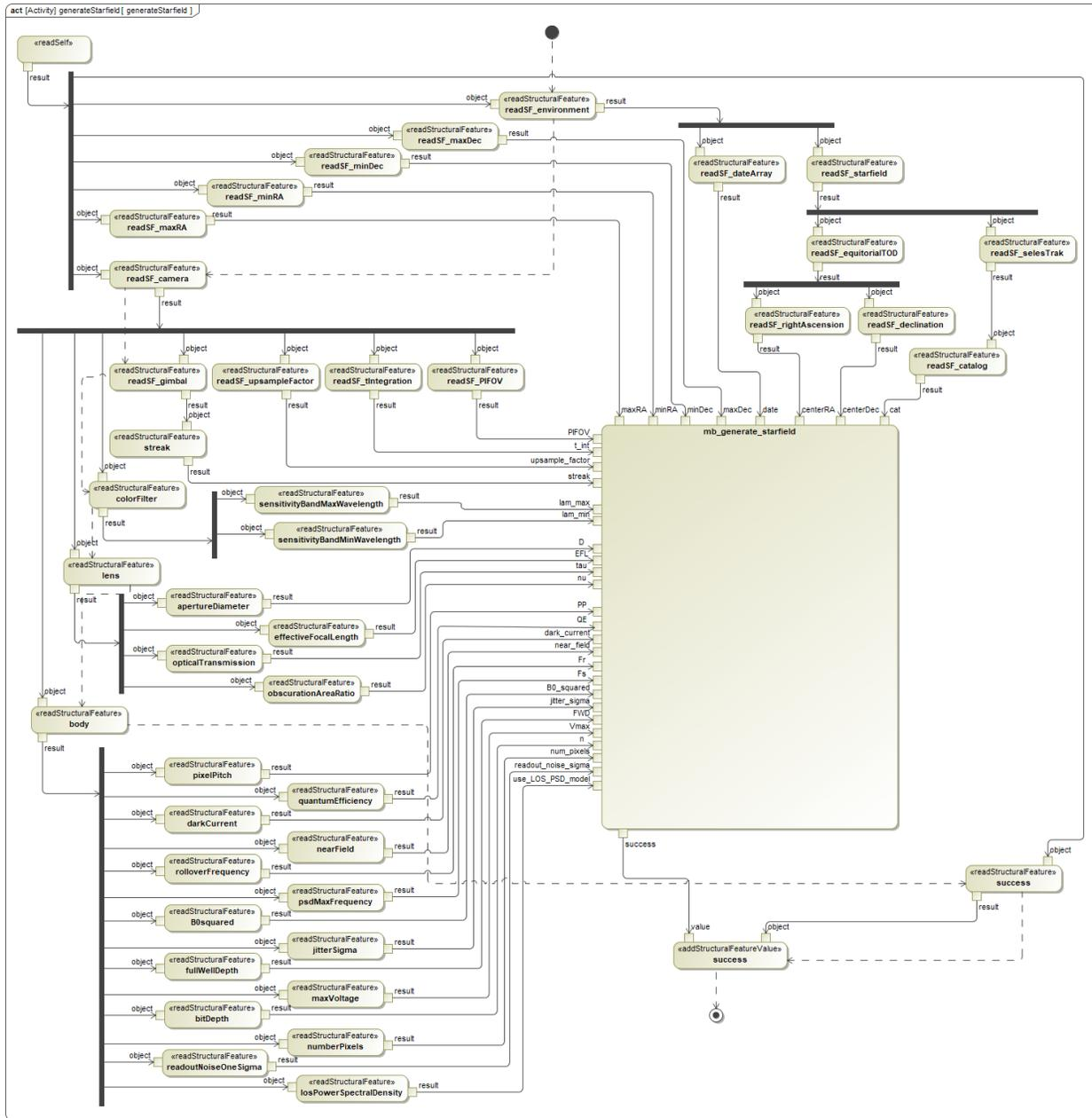
**Figure 9:** This activity diagram illustrates the complexity needed in an executable model. The inputs are pulled from calculated model constraints, as well as user selections for setting, filter, gimbal, and star catalog.
