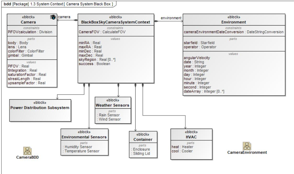
**Figure 2:** This diagram shows the base system components and model structure. Note, there are several elements not currently used in the analysis case presented in this paper.
