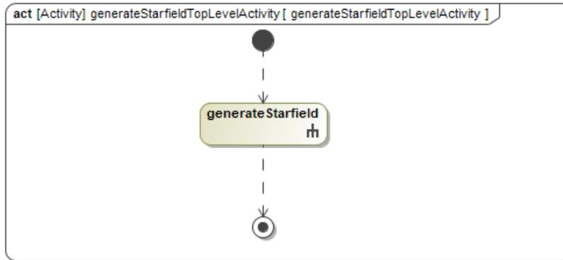
**Figure 8:** This is the top-level activity created by assigning an activity to the “do/” portion of the state machine `BlackBoxCameraSystemContext`.
