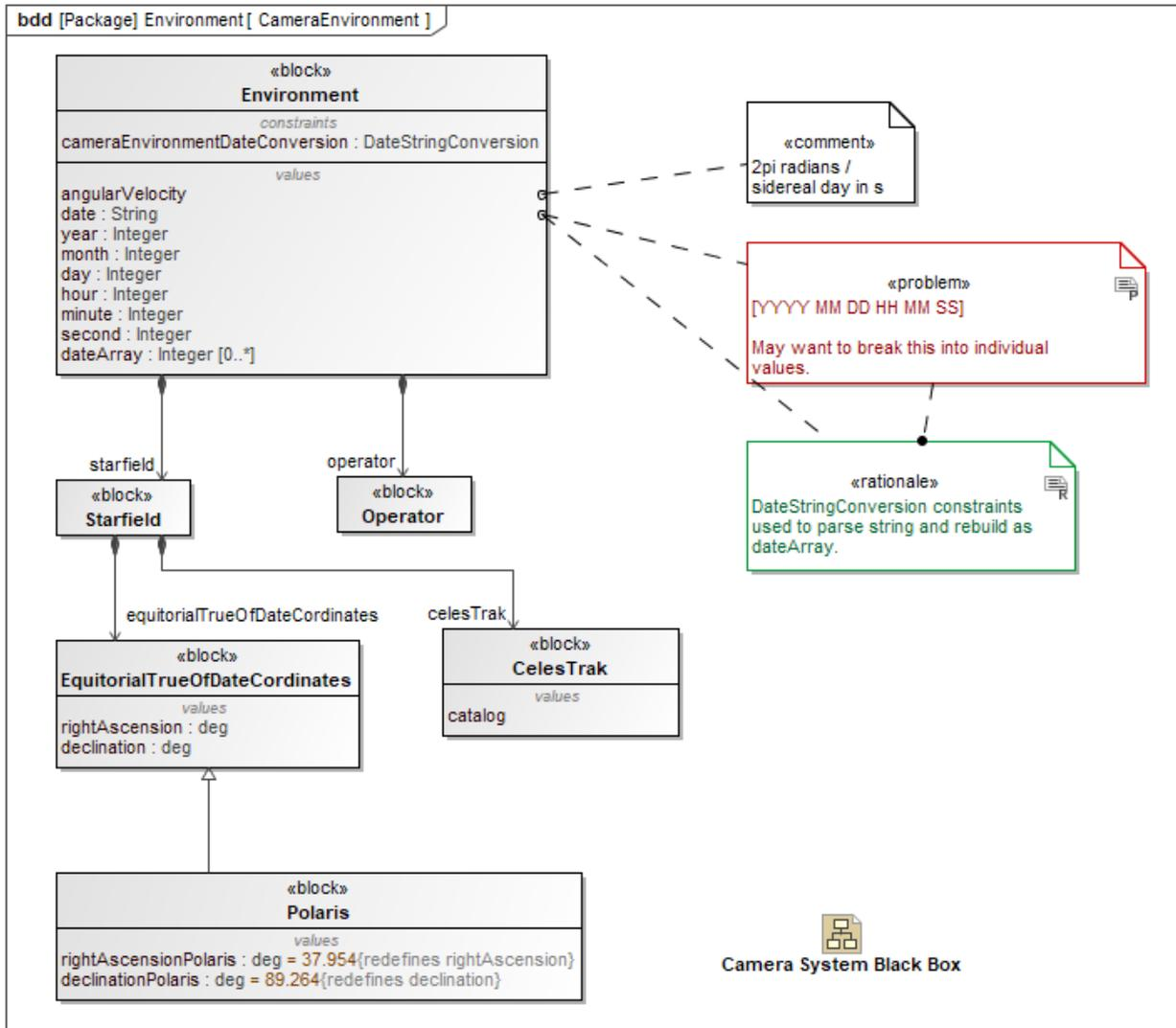
**Figure 3:** The environmental elements used in the model.
